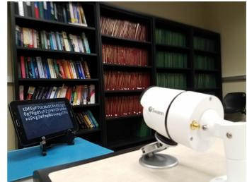
(c) Passphrase visual challenge being displayed on the field-of-view of a Swann 720p wireless IP camera with day/night vision and built-in cut IR filters.
