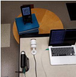
(a) Verifier code (running on laptop) sending visual challenges to a display in the field-of-view of a camera.
