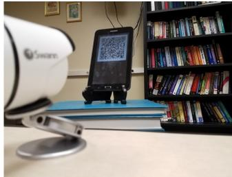
(b) QR code visual challenge being displayed on a small tablet device (i.e., independent from camera and verification mechanism).
